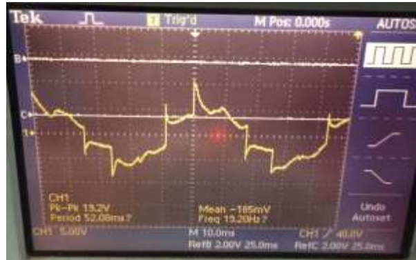
Figure 11 Output current waveform at lower motor speed
